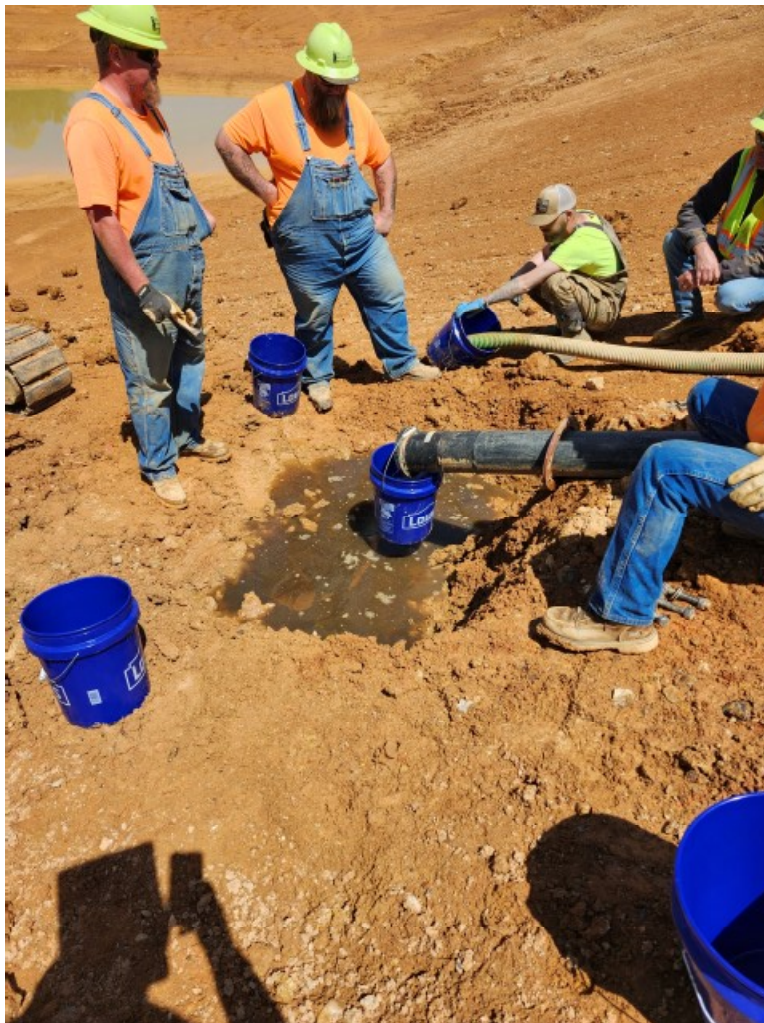
SITE PHOTO 4 – TYPICAL LEACHATE COLLECTION IN BUCKET BY HINKLE
